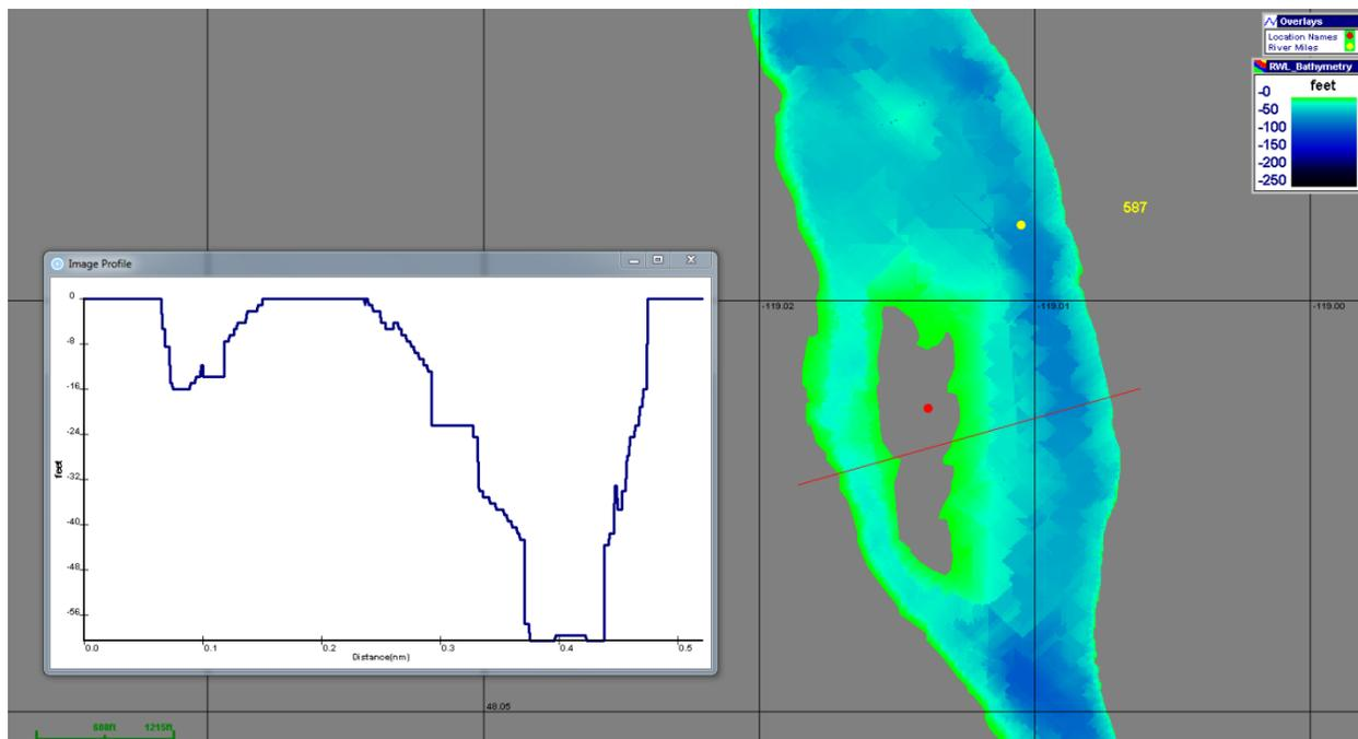
Figure 31. Zoomed-in image of Buckley Bar, with image profile window showing a 2D bathymetric transect along the thin red line bisecting the reservoir and Buckley Bar.
