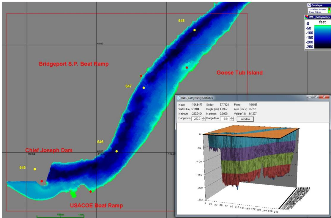
Figure 30. Zoomed-in image of lower Chief Joseph Dam pool, with image statistics window showing a 3D bathymetric profile of the area enclosed by the thin red rectangle.
