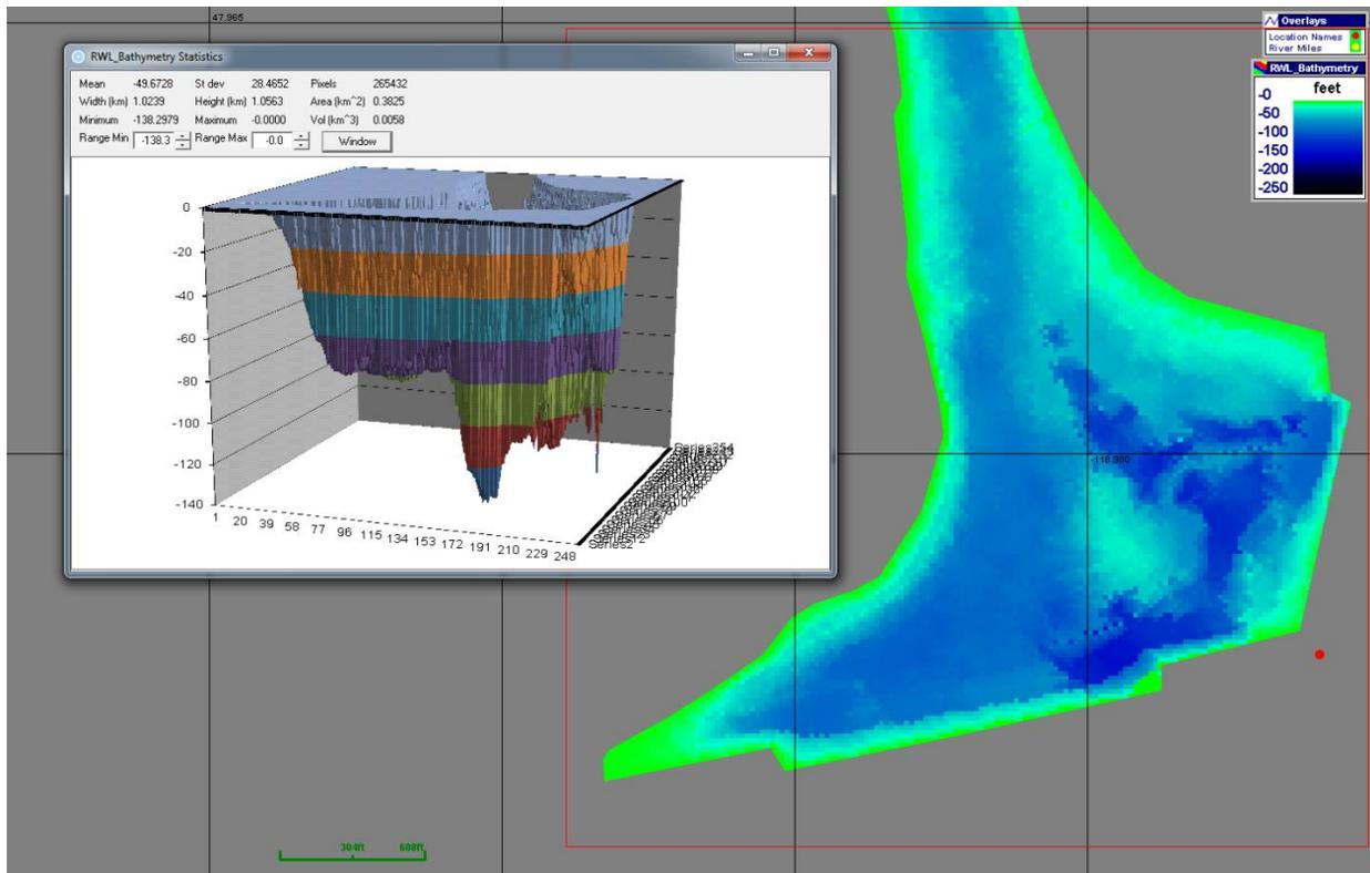
**Figure 32. Zoomed-in image of Grand Coulee Dam tailrace, with image statistics window showing a 3D bathymetric profile of the area enclosed by the thin red rectangle.**
