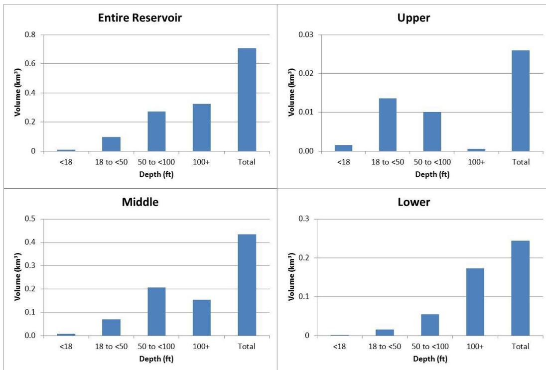
Figure 34. Volume estimates for different sections and depth strata of Rufus Woods Lake, calculated with Environmental Assessment System (EASy). Same note from prior figure applies here.
